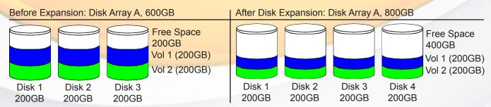
The RAIDBank4 controller redistributes the original volume set over the original and newly added disks, using the same fault-tolerance configuration. The unused capacity on the expanded RAID set can then be used to create additional volume sets, with a different fault tolerance setting if required.
